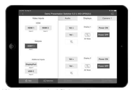
Output names entered in KDMS Pro are visible at the top-center of each Display control button group.
