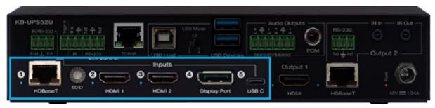
**HDBaseT** (Input 1): Using a CAT5e/6 cable, connect from a compatible KD Transmitter.
