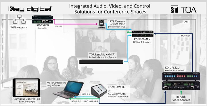
**Products shown:** TOA <u>Lenubio</u>, VISCA RS-232 PTZ Camera, Key Digital <u>KD-X4x1WUTx</u>, <u>KD-UPS52U</u>, <u>KD-CamUSB</u>, <u>KD-CX800</u>, <u>KD-ProCL1</u> **System Delivery:** Connect laptop USB and AV to present and provide remote participants an HD 1080p professional auto-PTZ controlled view of the conference space while speaking with each other just as they would in normal conversation thanks to the integrated array mic and soundbar.
