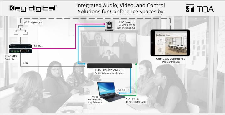
**Products shown:** TOA Lenubio, VISCA RS-232 PTZ Camera, Key Digital KD-CX800, KD-Pro16, KD-Pro16, KD-ProCL1 **System Delivery:** Connect laptop USB & HDMI to present and provide remote participants an HD 1080p professional auto-PTZ controlled view of the conference space while speaking with each other just as you would in normal conversation thanks to the integrated array mic and soundbar.
